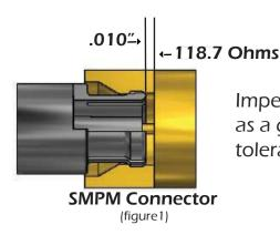
Impedance changes in a typical SMPM coaxial connector interface as a gap is introduced due to typical and expected mating tolerances (see figure 1)
