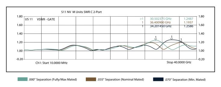
The PkZ provides a constant impedance profile over wide gaps in the mating interface, thus minimizing negative impact on VSWR.
