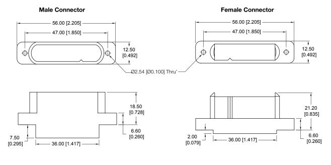
Removable contacts should be allowed to float after installing in connector body for optimum mating. Consult Technical Sales if alignment insert for male contacts is desired. Alignment insert for GFSH89, GFSH109 and GFSH928 are available. Consult Technical Sales for other versions.
