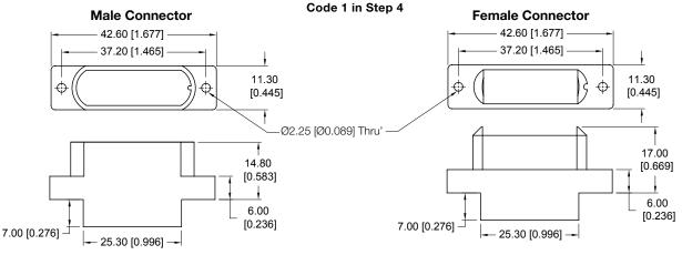
Removable contacts should be allowed to float after installing in connector body for optimum mating. Contact Technical Sales for additional polarization features for panel mounting.
