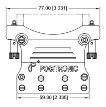
Code W: Hood, cable clamps, hex nuts and screws. Code WE : Hood, rotating jackscrews, cable clamps, hex nuts and screws.
