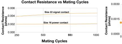
Humidity condition per EIA-364-31B, Method II (condition A) after 250, 500 and 1,000 cycles. Contact resistance tested per IEC 60512-2, Test 2b. Connectors tested: GFSH624.
