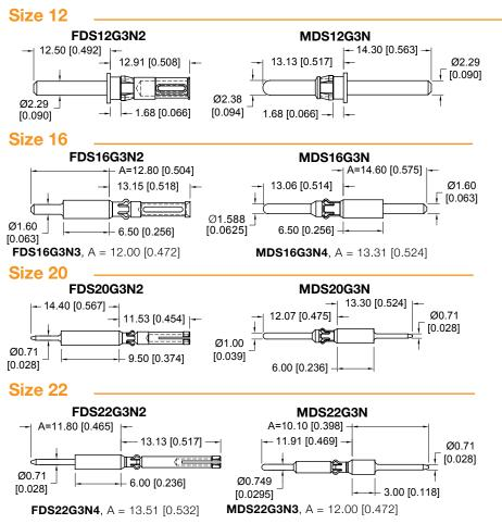
**Material and Finishes:** Precision machined copper alloy with gold flash over nickel. Other finishes are available.
