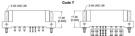
Note: For GFSH624, only PCB male fixed jackscrew and Panel female rotating jackscrew is available.
