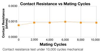
operation using GFSH89 with 12 AWG wires and size 16 contacts under load (not utilizing signal contacts). Tested per IEC 60512-2, Test 2b. Connectors tested: GFSH89.
