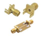
GigaLane End Launch SMA Connector is designed for applications such as High Performance RF Circuit Boards. It is attached to RF circuit board by inserting the board edge between legs and soldering legs. It has excellent return Loss up to 26.5 GHz.
