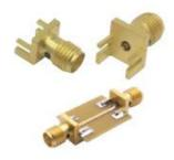
GigaLane End Launch SMA Connector is designed for applications such as High Performance RF Circuit Boards. It is attached to RF circuit board by inserting the board edge between legs and soldering legs. It has excellent return Loss up to 26.5 GHz.
