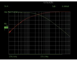
Typical Low Frequency Insertion Loss (red) and Return Loss (green) measured on K251 over the range of 1kHz to 1 MHz.
