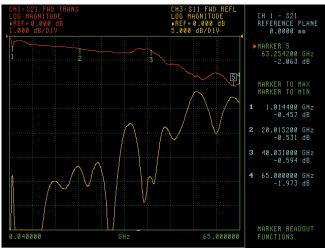
Typical Low Frequency Insertion Loss (red) and Return Loss (yellow) measured on V251 over the range of 40 MHz to 65 GHz.
