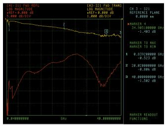
Typical Low Frequency Insertion Loss (yellow) and Return Loss (red) measured on K251 over the range of 40 MHz to 40 GHz.
